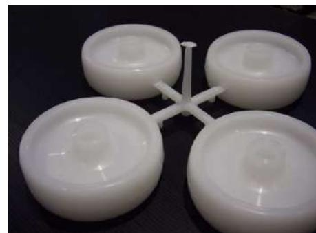
*We carry out the injection processes for castors and castors components with all the plastic materials we use: nylon, polypropylene, polyurethane, polyethylene, nylon with fiberglass, polycarbonate ...*
